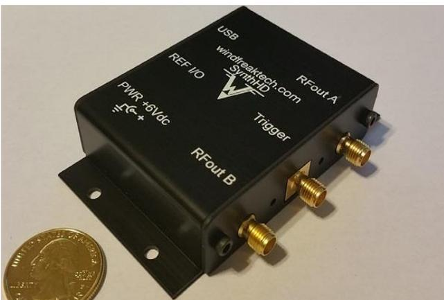
The SynthHD has powerful software and firmware features such as sweeps, lookup table frequency and amplitude hopping, pulse modulation, AM, FM and FMCW pulsed chirps. Experiment with dual super-het LO generation, quadrature LO generation, antenna beam steering and more. The SynthHD is a great addition to test equipment either in a lab environment or as a highly portable device used in the field. Also, the SynthHD works well as a basic building block in microwave communications systems.
